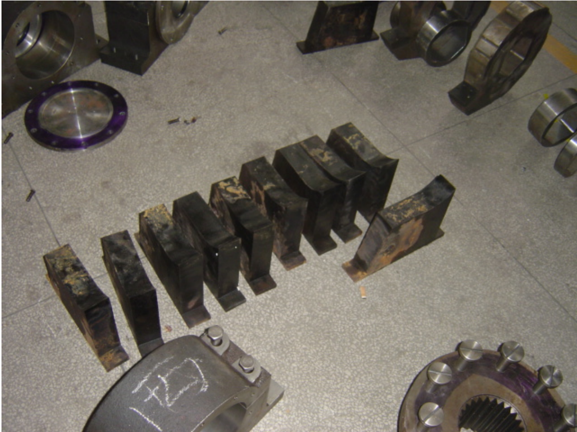
This is a photo of the cleaning fingers for a unit and some of the other parts associated with our new series of shredders. Lower left is the top cover of the bearing assembly. Lower right is one half of the torque coupling and its torque bolts. Note the splined shaft in the coupling for added strength.
