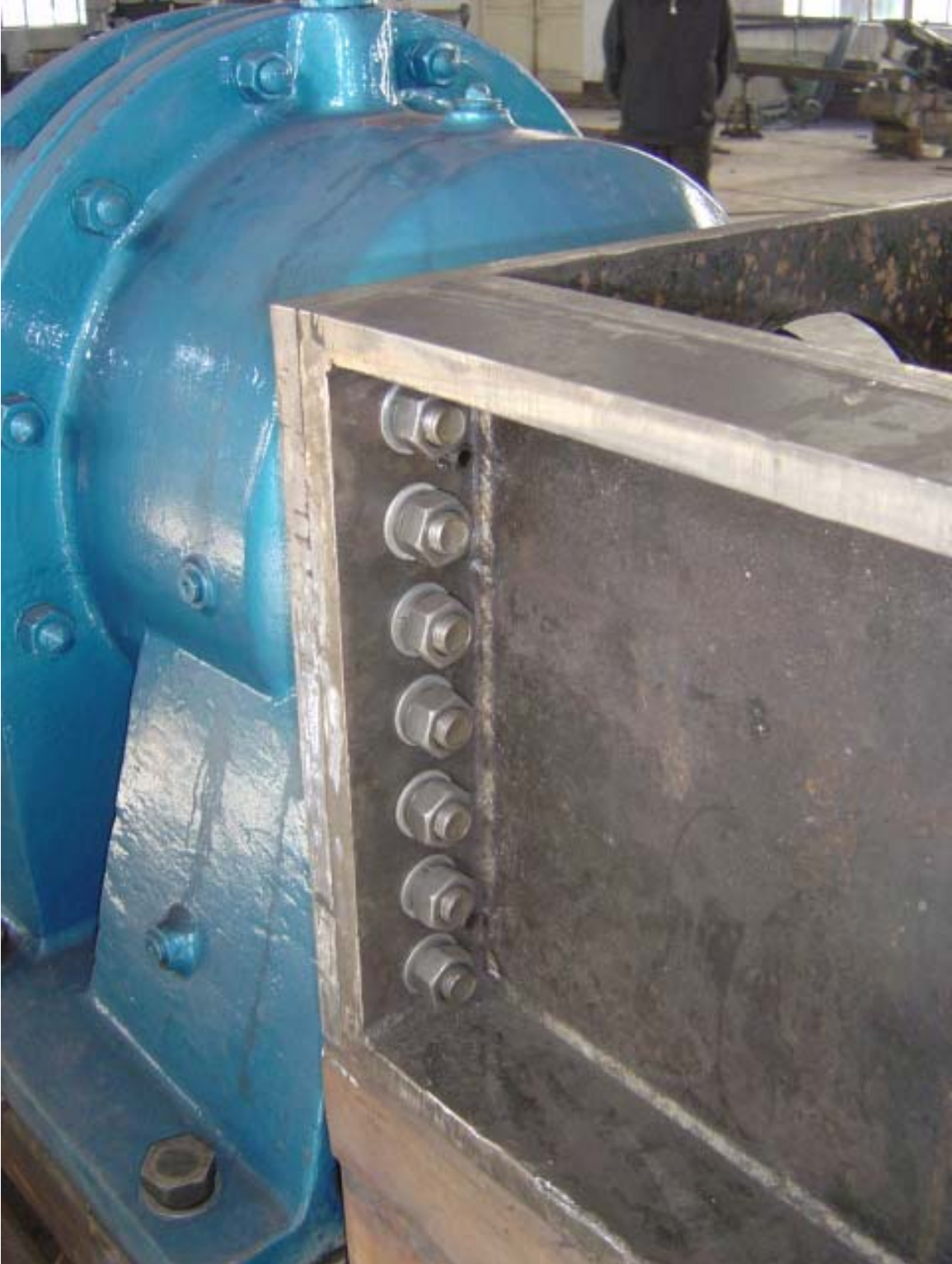
Another Picture of the 7 bolts that can be removed from each end of the shredder allowing for a total removal of the entire side plate of the shredder for fast and easy replacement of an entire cutter assembly.
