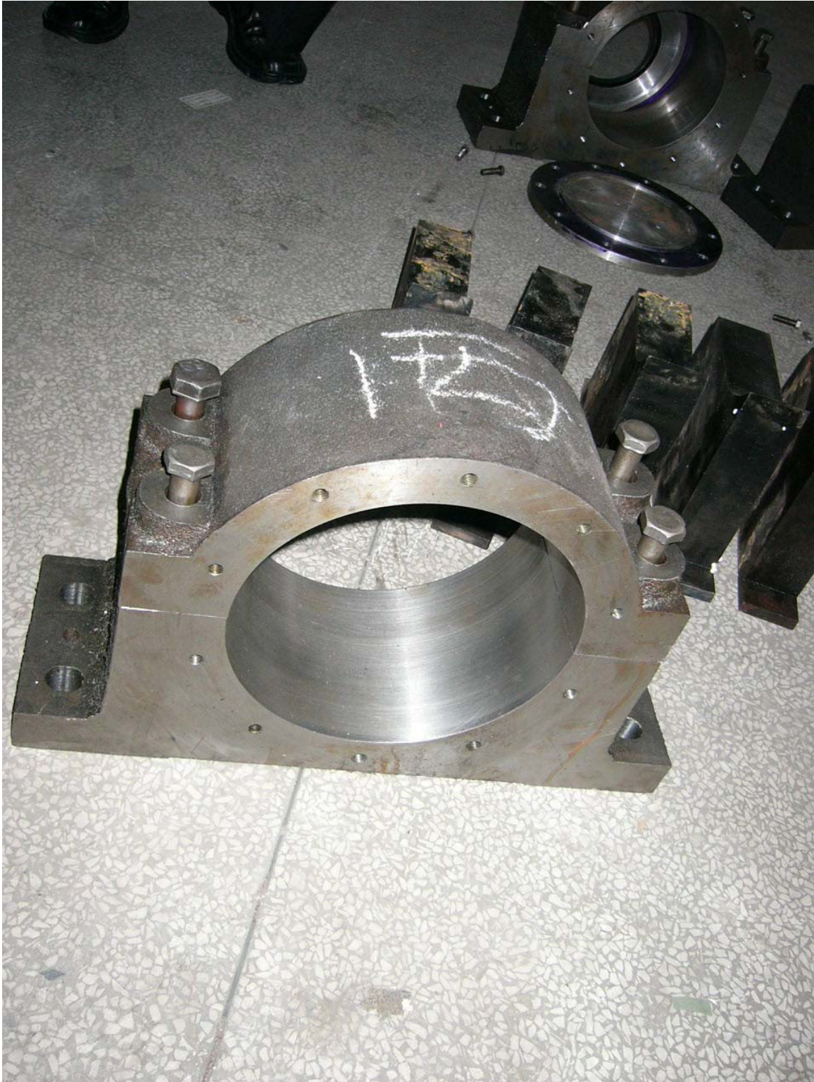
This picture shows one of four solid steel castings for the bearing housings. They are split so to allow for removal of the bearings from the housing without using a pulling type design common to most shredders in the industry today. The old designs that we pioneered in the early 1970's
