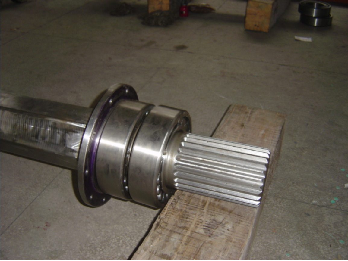
This is the splined drive end of a shaft also showing the double bearing design of our shredders. Material is a heat treated 4140 allow steel.
